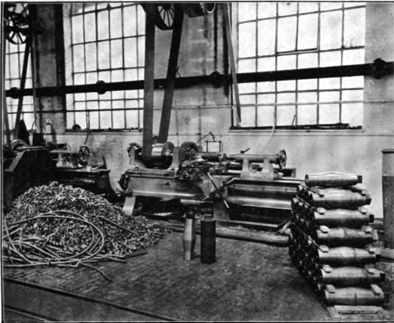
A. Turning armour-plate bolts with "A. W." high-speed steel. One day's work of 10 hours is shown, 40 bolts being turned in that period. Cutting speed, 160 feet per minute; maximum depth of cut, \frac{3}{8} inch; feed, 32 cuts per inch; weight of metal removed from each bolt, 62 lbs.; total weight removed, 2480 lbs. (Sir W. G. Armstrong, Whitworth & Co., Ltd., Manchester.)
